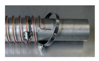
9. Push the wire connection clamp and the hose onto the pipe
