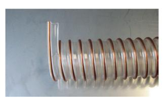
4. Peel the end of the wire, so that it is free from the wall material. Remove the plastic with a sharp instrument. Please ensure that you cut away from your body, in order to avoid any injuries.
